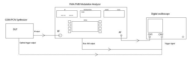
FIG. 3: Test setup for transient measurements
